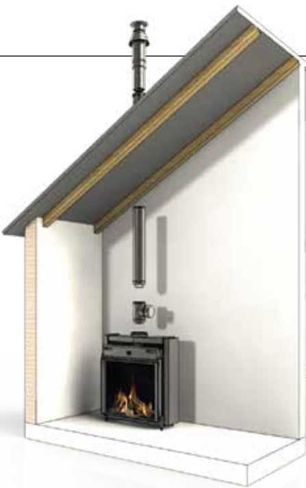
Via roof [pitched] • straight or with bends
